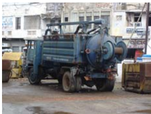
Sewer line cleaning machine (Picture – Morbi city)
