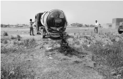
Disposal of untreated wastewater and septage
