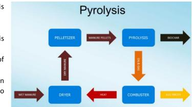
produce complex oil in the absence of air/oxygen. In this technology sludge is converted to Bio-oil, Pyrolytic Gas and Bio-char. Here also drying of sludge is required prior for treatment in incinerators. This technology requires trained operators and there is risk of malfunction if not properly maintained and operated.
