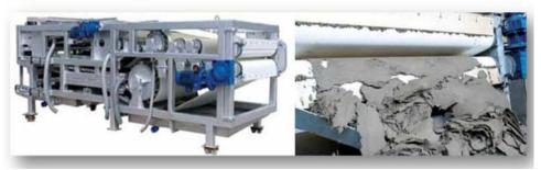
Both solid and liquid parts still contain pathogens and pollutants and further treatment is necessary. Mechanical parts need periodical inspection and replacement.
