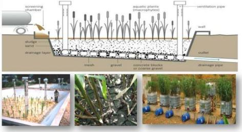
systems that maintain the porosity of the filter. The roots of the plants create pathways through the thickening sludge to allow water to escape more easily.
