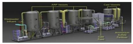
In this technique black water, faecal sludge and grey water is converted to fertilizer and treated waste which can be use in agriculture, arboriculture, pastures, ground water recharge in deep aquifer and desert areas. This technology is highly expensive.
