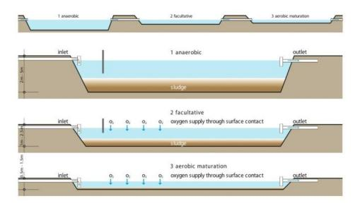
As per sanitation experts and review of various technical documents, it was analysed that waste stabilization pond is good option for treatment of wastewater but not a good option for treatment of Septage.
