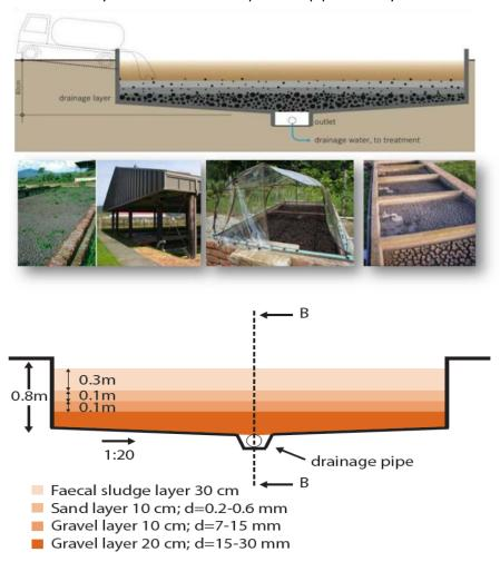
gravel that support the sludge and allow the liquid to infiltrate and collect in the pipe.
