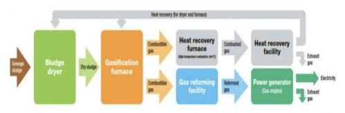
**Advantages:** Technology best suitable for dry feed stocks. The produced gas can be converted into any type of fuel by FT synthesis.
