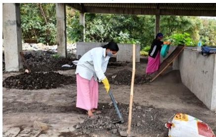
The women sanitation worker mixing and rotating dried sludge on platform
