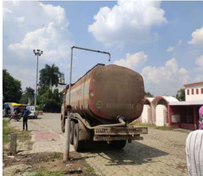
Figure: Tanker getting filled by treated wastewater from hydrant
