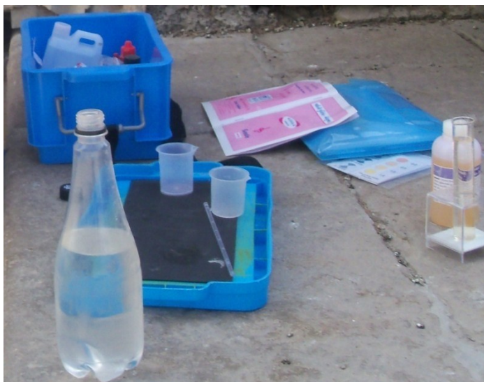
Photograph 2 Kit for testing water quality in field
