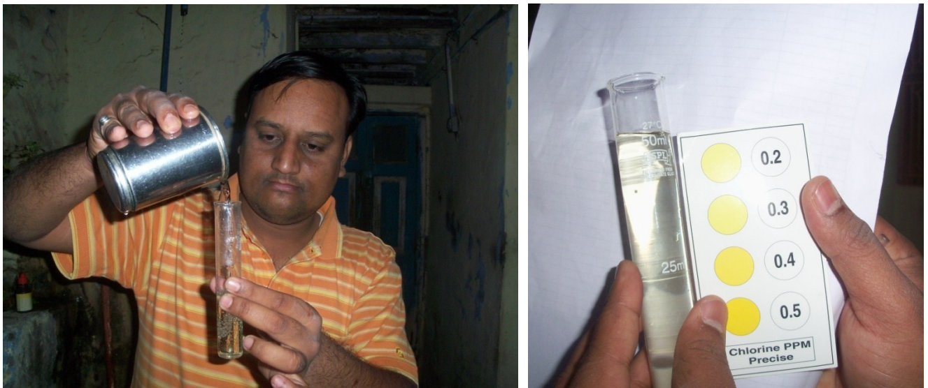
Photograph 3: RC testing on site
