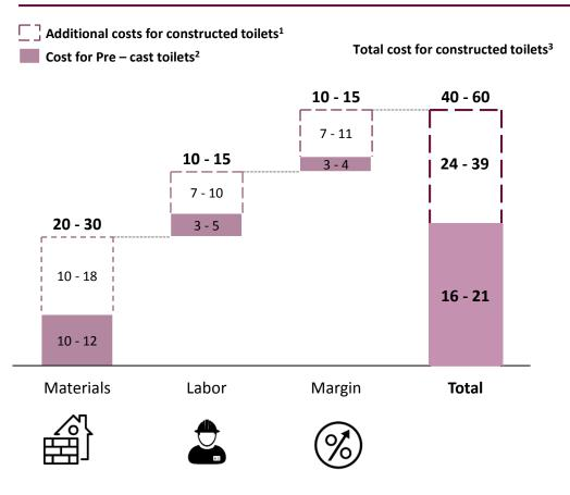
Pre-cast toilets with cylindrical septic tanks are better since they can be made faster and are cheaper than normally constructed toilets – Pre-cast contractor in Sinnar
