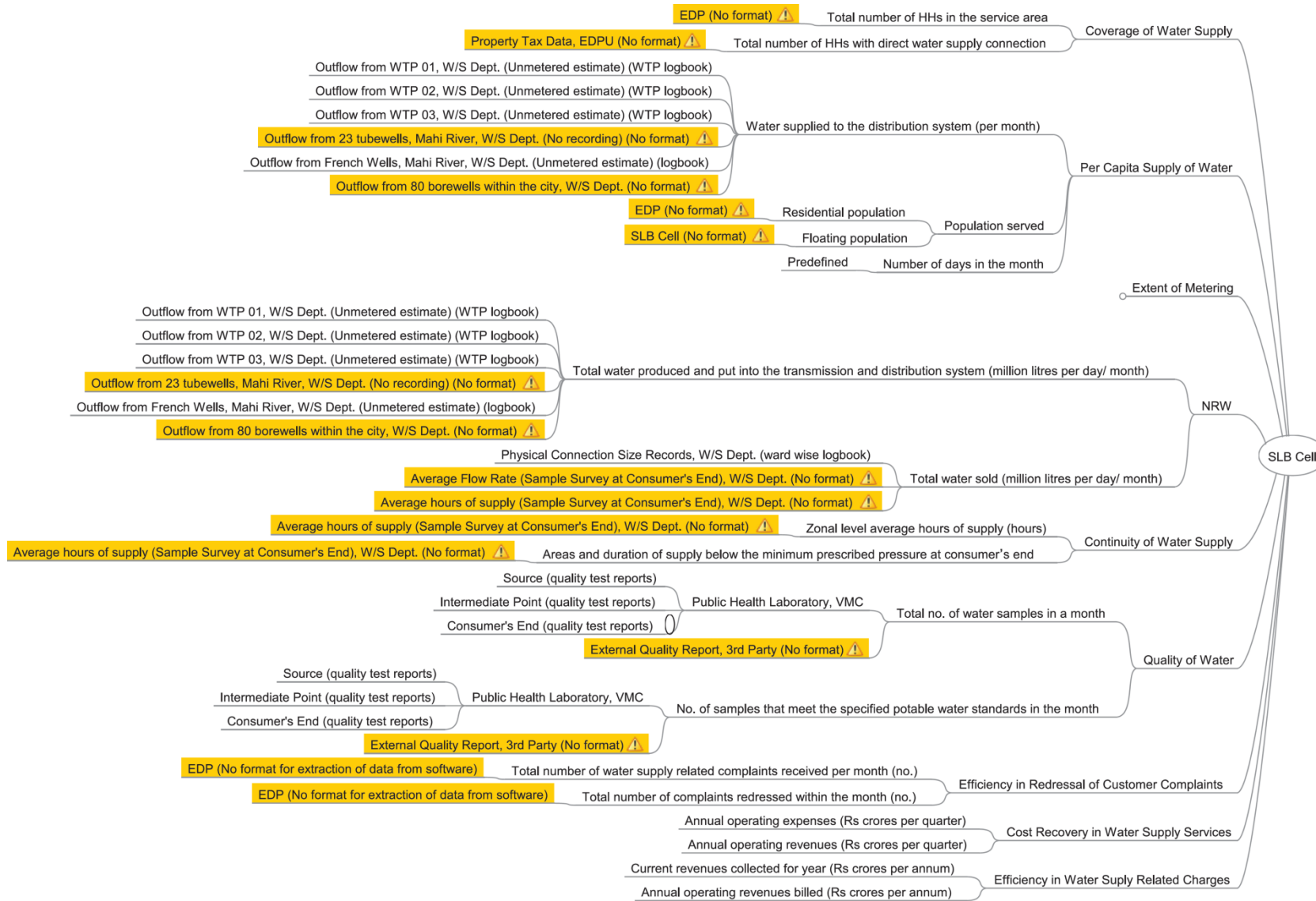
Figure 5 Information flow diagram for calculating water supply related performance indicators as per SLB framework
