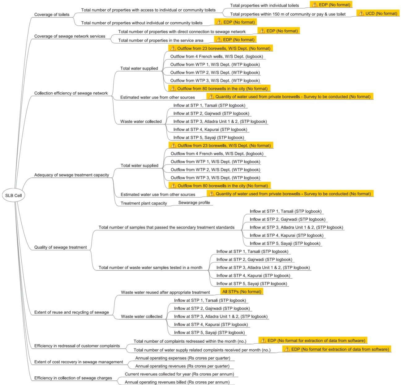
Figure 13 Information flow diagram for calculating sewerage related performance indicators as per SLB framework
