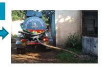
Desludging Trucks visits the Jayanti Nala Pumping Station or Dudhali pumping Station for discharge the septage
