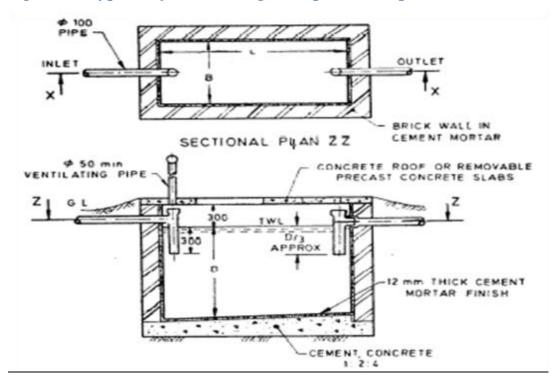
Figure A2: Typical layout for a double compartment septic tank for 50 users
