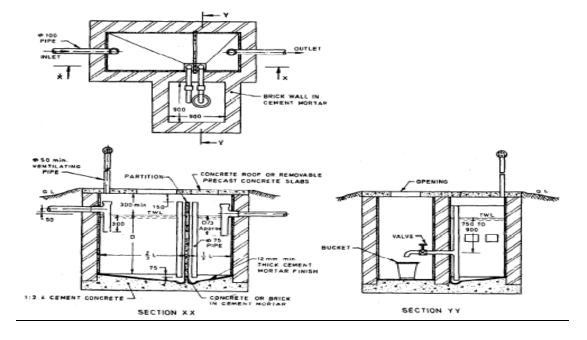
Figure A3: Typical layout for a double compartment septic tank for more than 50 users
