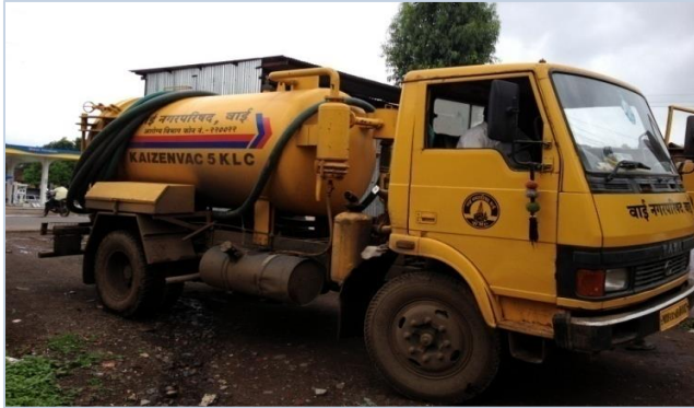
Suction truck of 5KL capacity in Wai
