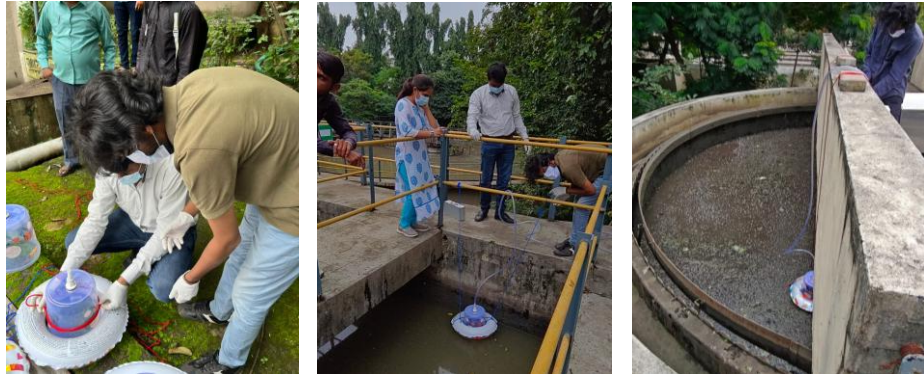
Figure 3 Flux chamber placement and sampling at different STP components
