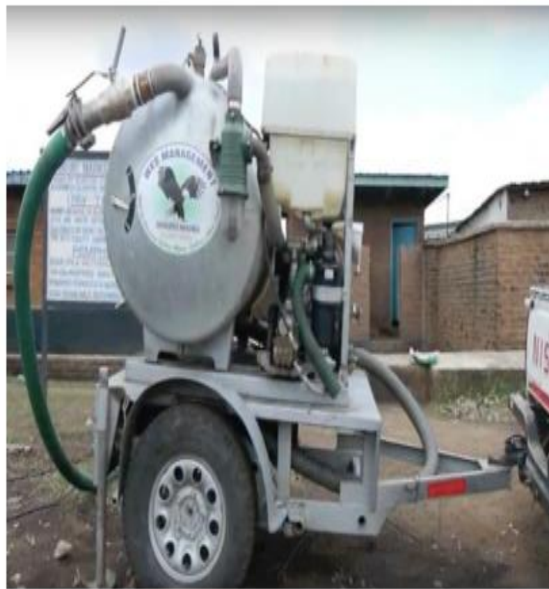
Mechanical De-sludging Units
