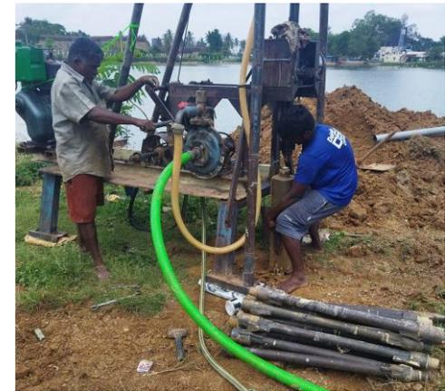
05. Green Pipe is the inlet from storage tank. Black and yellow hose pipe is outlet from drilling machine to circulate the water
